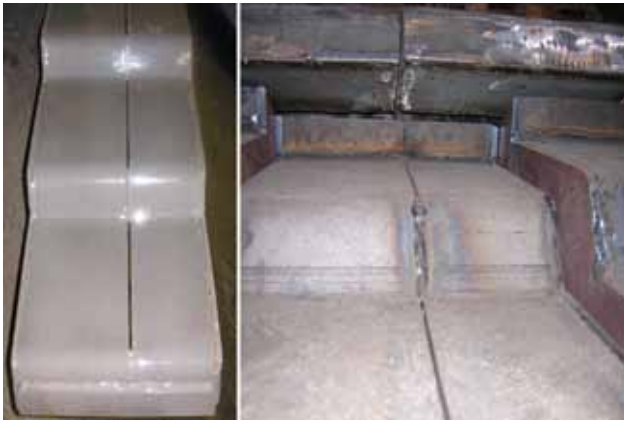
300 mm grate block. Note the air gap and side section
