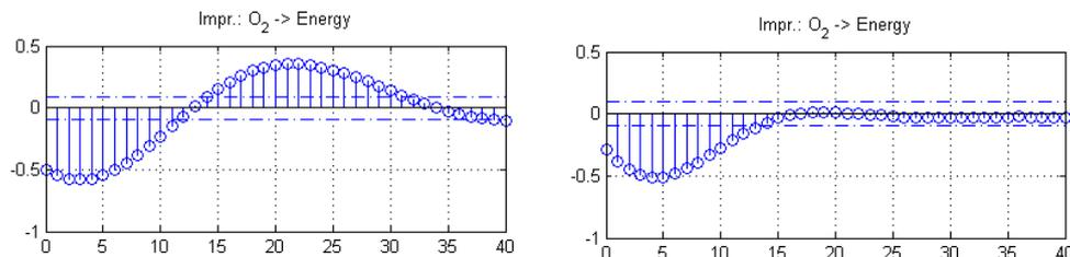
Figure 6. The left sub-plot shows the impulse response function with oxygen as input and steam production as output for the old PID structure. The right sub-plot shows the same, but for the new PID structure. The Y-axis shows the size of the coefficient (normalized data) and the X-axis the time lag in minutes.
