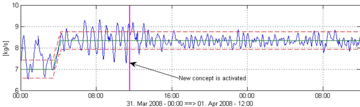
Figure 4. The new concept is activated. The green line is the set point. The blue line is the actual steam production. The red lines are +/- 5% of the set point.
