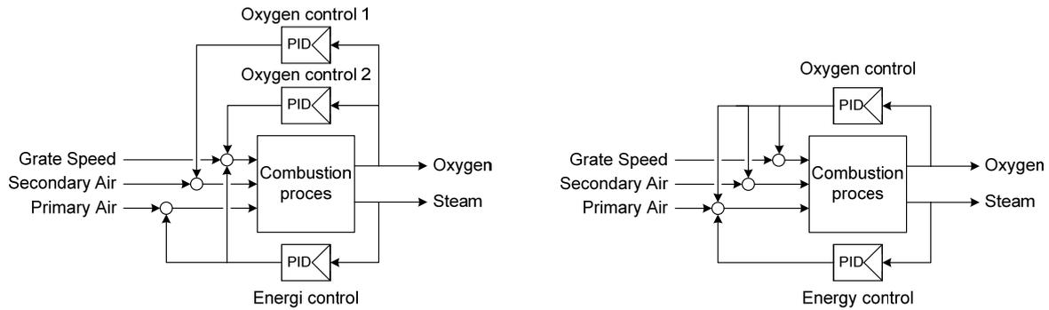
Figure 3. The left figure shows the PID structure commissioned in 2005, referred to as the old PID structure. The figure to the right shows the improved PID structure activated in the spring of 2008, referred to as the new PID structure.
