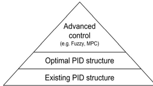
Figure 1. The control strategy upgrading triangle.
