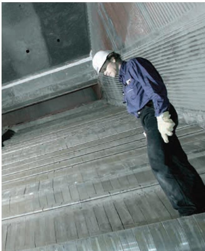
DynaGrate® seen from ash outlet. Feeding pusher inlet is at the top of the grate.
