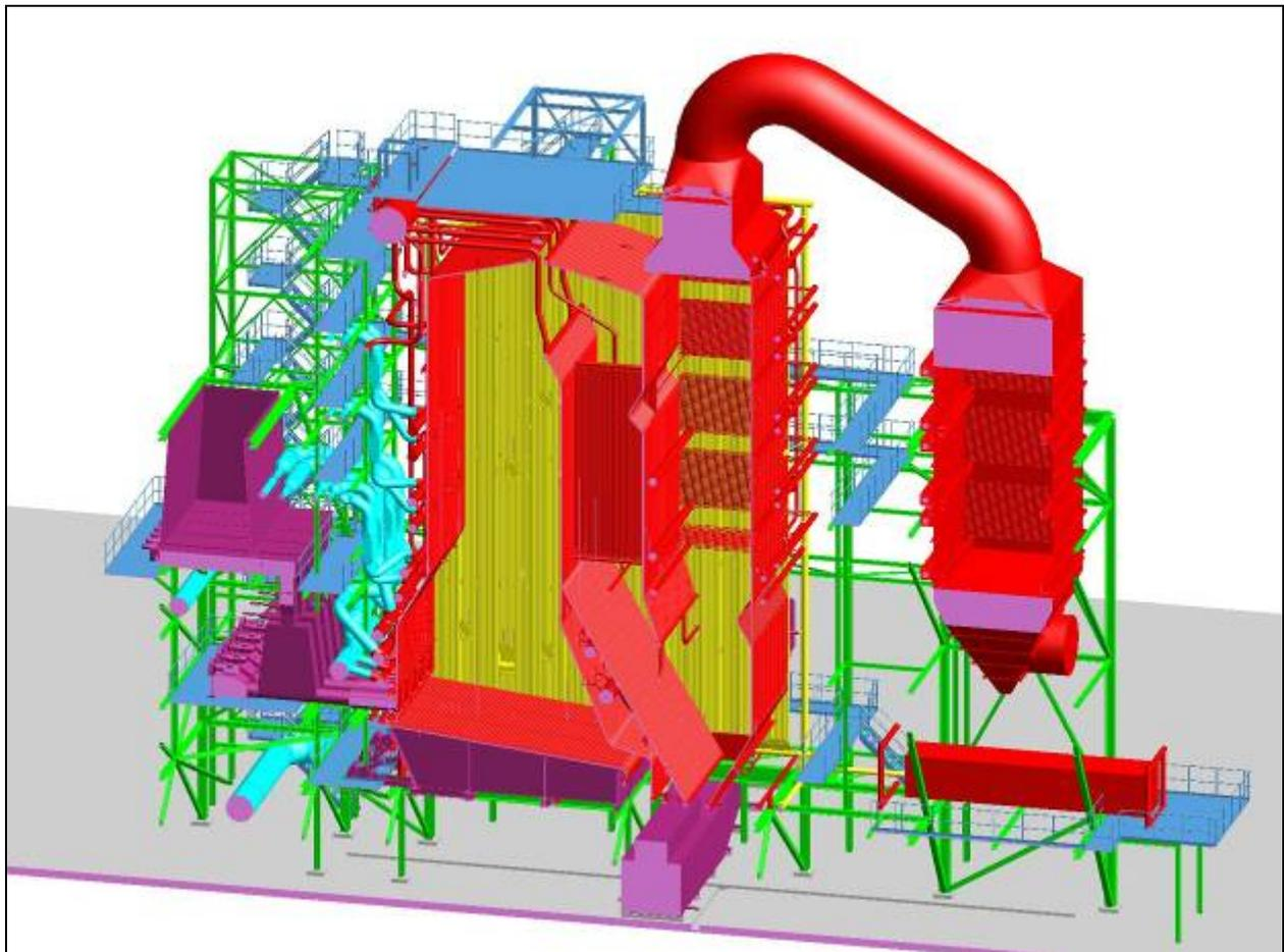
Figure 3. Plant layout for the bran fired boiler at Biowanze, Belgium.
