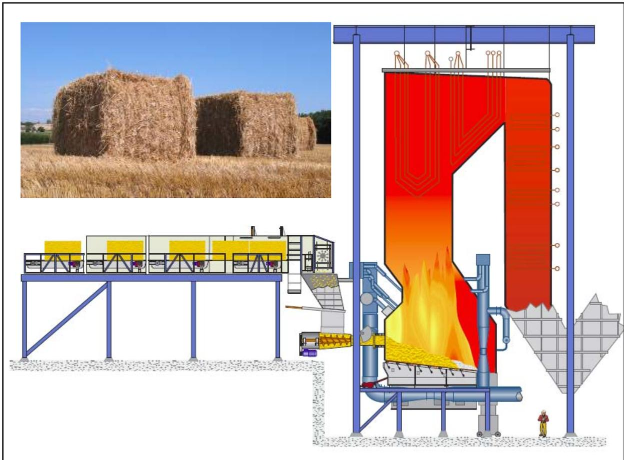
Figure 1. Fuel pre-treatment system and boiler for the 105 MW<sub>th</sub> ultra super critical unit.
