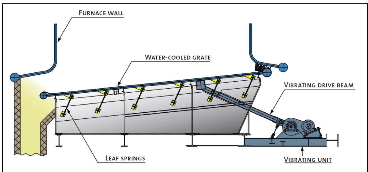
Figure 2. Babcock & Wilcox Vølund's water cooled combustion grate.
