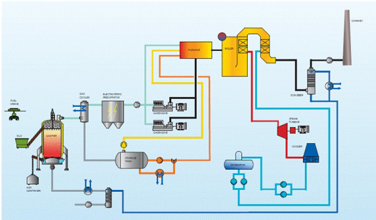
Figure 3: A combined cycle gasifier-based power plant (CC-CHP).
