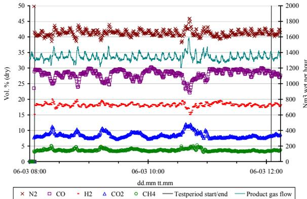
Figure 3. Composition and flow of product gas during the performance test.
