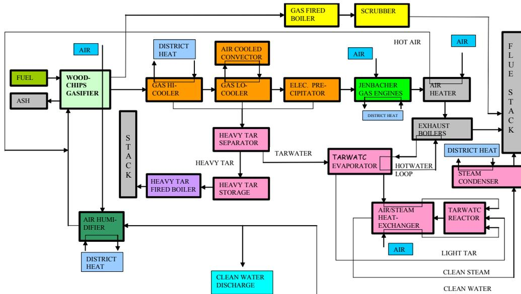
Figure 2. A schematic drawing of the Harboøre CHP plant.
