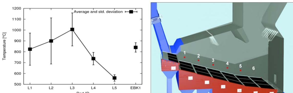
**Figure 3** Temperature measurements, Concentration of CO, CO<sub>2</sub> and O<sub>2</sub> along ports L1-L5 and in first draught (EBK1).
