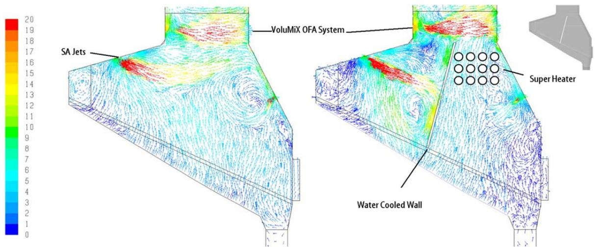
Figure 5 Velocity [m/s] vector plot, in a plane with jets, close to the centre of the furnace.
