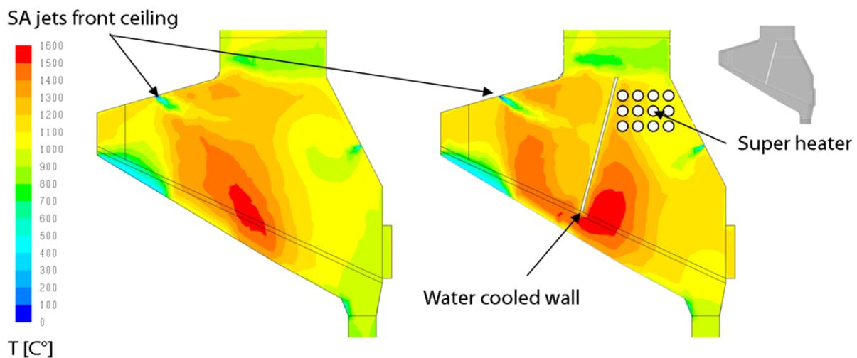
Figure 6 Gas temperature distributions in the centre of the furnace.
