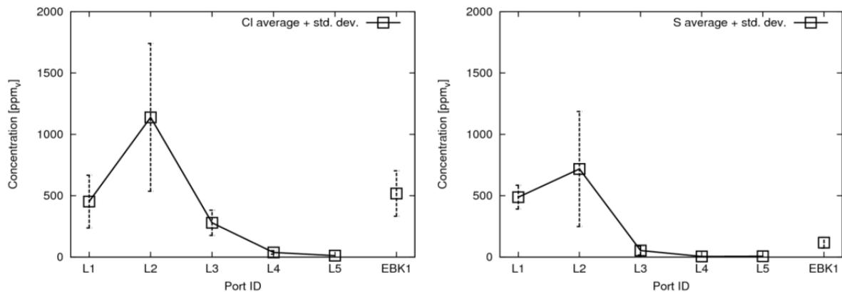
**Figure 4** Chlorine and sulphur concentrations at ports 1-5.
