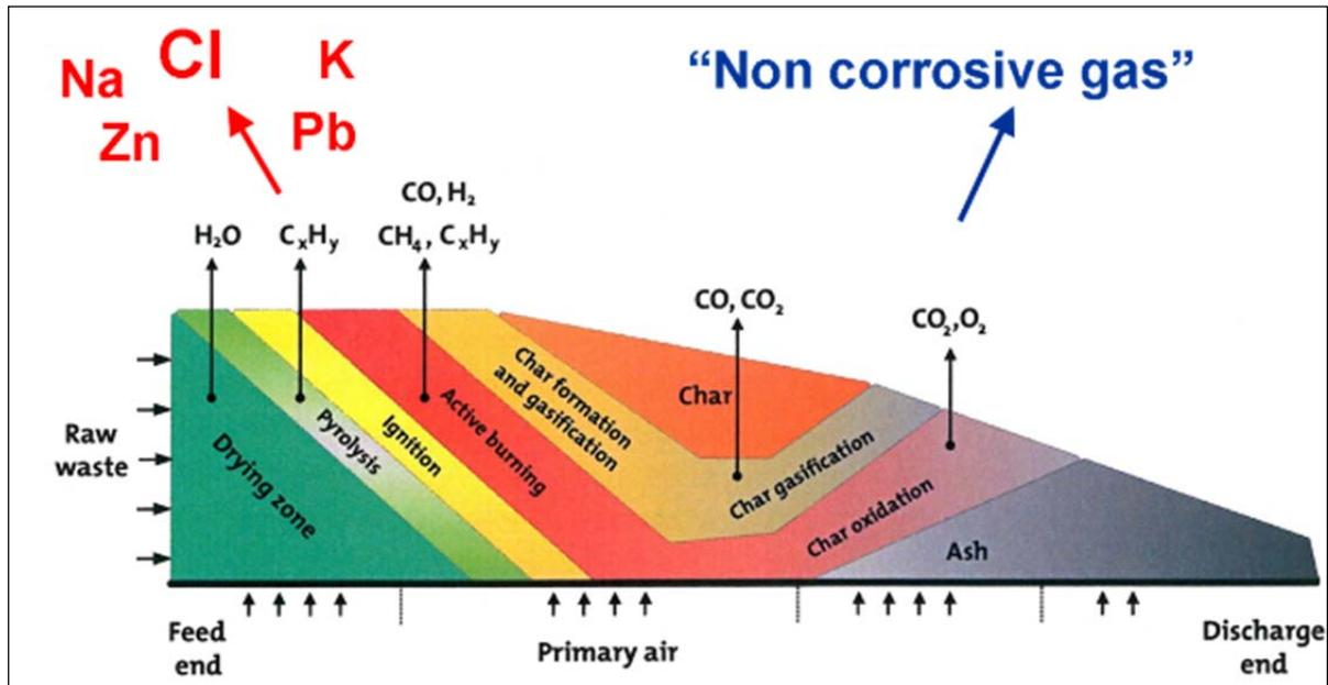
**Figure 1** Schematic view of the fuel bed combustion process and the potential release of the volatile elements Cl, Na, K, Pb, Zn and S to the flue gas in the first part of the furnace.
