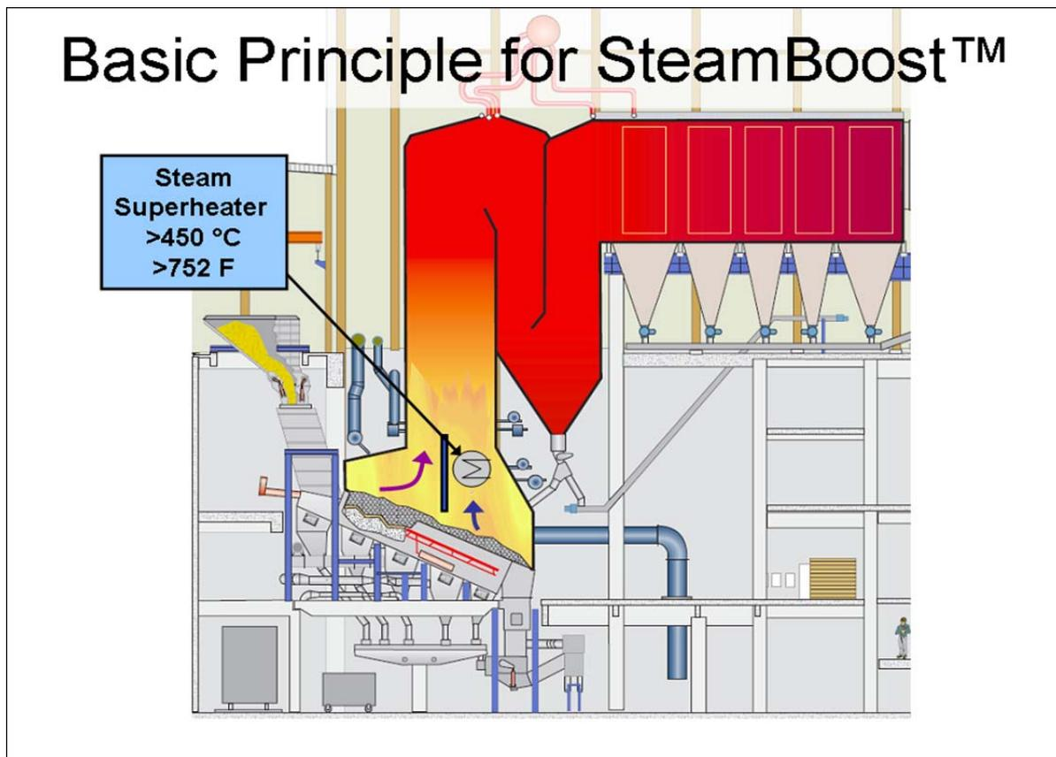
**Figure 2** Generic waste fired power plant with two-stage furnace and SteamBoost™ super heater.
