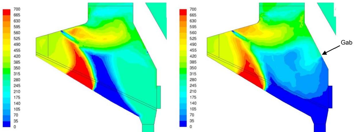
**Figure 7** Chlorine [ppm] concentration profiles before and after changing the flow field.
